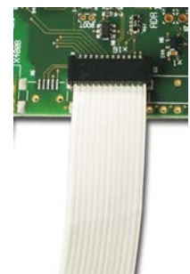
Figure 59: Connecting the Diagnostic detached Network Interface (AIFX-DIAG) to the Basic Card CifX 104C-FB-R\F (Example)
