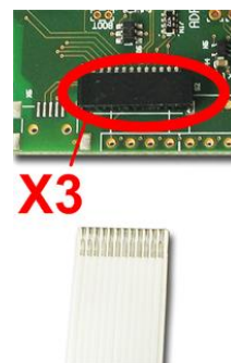
Figure 59: Connecting the Diagnostic detached Network Interface (AIFX-DIAG) to the Basic Card CifX 104C-FB-R\F (Example)
