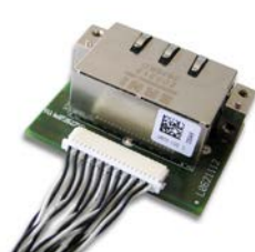
Figure 57: Connecting the Detached Network Interface Ethernet (AIFX-RE) to the Basic Card CIFX 104C-RE\F (Example)
